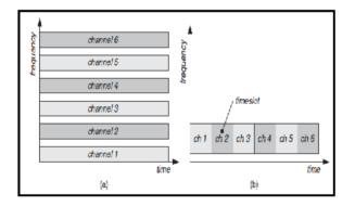
Figure 2: Frequency and Time Division Multiple Access
