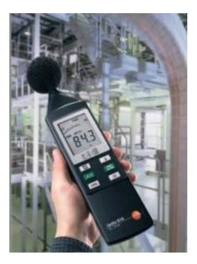
Figure (3): Sound pressure level meter.
