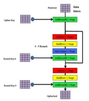
Figure 1. Block Diagram for the AES Structure.
