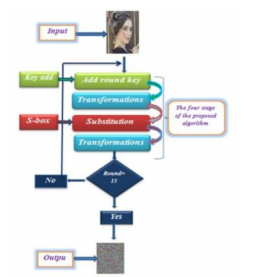
Figure 2. Block Diagram for the proposed algorithm
