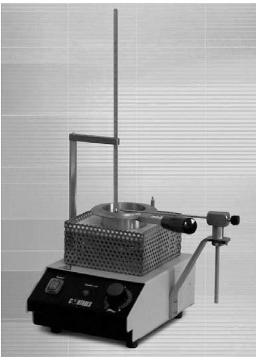
Figure 18.10 Apparatus for Cleveland Open-Cup Test
