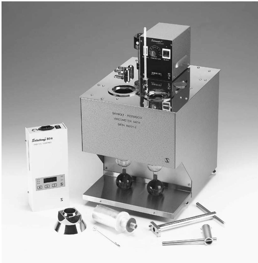
Figure 18.2 Saybolt Furol Viscometer
