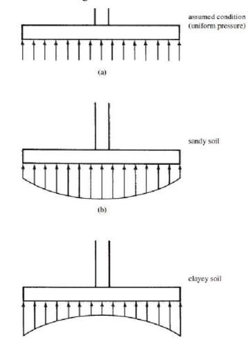
Just the opposite situation is true for footings supported by clayey soils. The clay under the edges of the footing sticks to or has cohesion with the surrounding clay soil. As a result, more of the load is carried at the edge of the footing than near the middle. The designer should clearly understand that the assumption of uniform soil pressure underneath footings is made for reasons of simplifying calculations.
