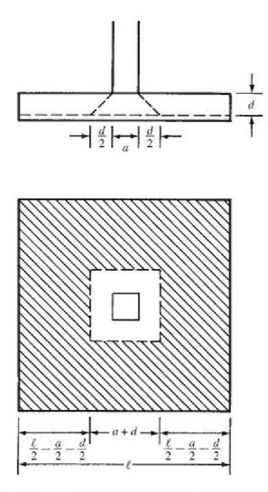
**11.11.2.1** — For nonprestressed slabs and footings,  $V_c$  shall be the smallest of (a), (b), and (c):
