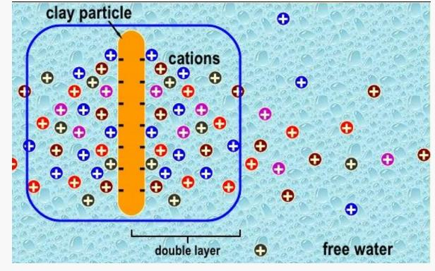
The electrically attracted water surrounds the clay particle is known as the diffused double-layer of water.
