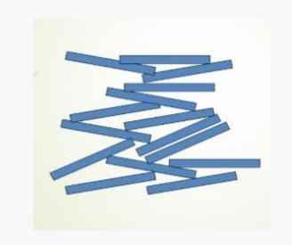
If there is net attraction the orientation of the particles tends to be edge-to-face or edge-to-edge, this being referred to as a **flocculated structure**.
