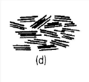
Assemblages can also occur in the form of connectors or a matrix between larger particles.
