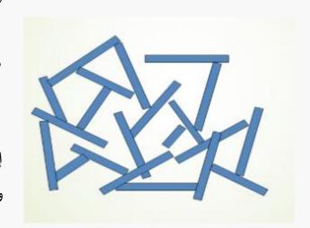
In natural clays, which normally contain a significant proportion of larger, bulky particles, the structural arrangement can be extremely complex.
