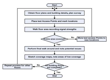
Figure 5: Flow Chart Explains Wireless Site Survey and Planning
