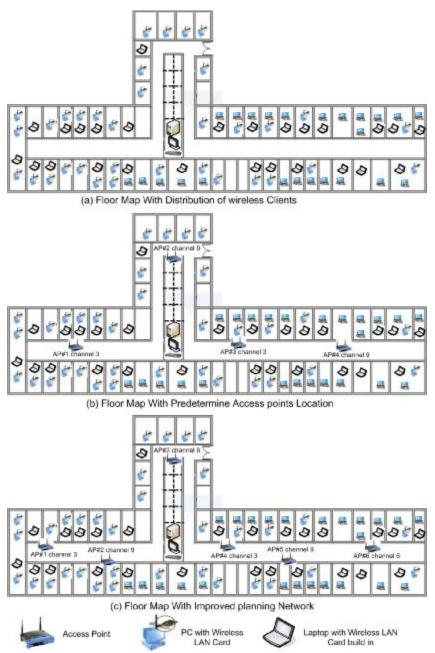
Figure 6: Implementation of Indoor Wireless LAN Network
