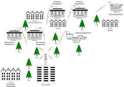
(a) Outdoor Wireless LAN Networks Using one Access Point Bridge and Omnidirectional Antenna
