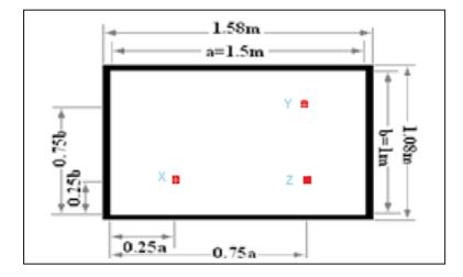
Fig.5. Schematic of the plate with cantilever configuration for the purpose of development of AVC
