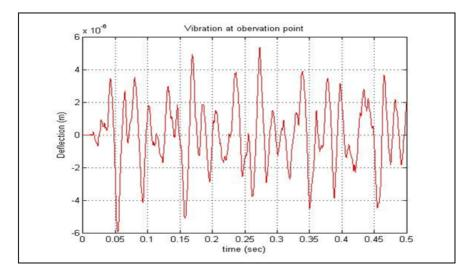
Fig.8. Lateral deflection detected at x=0.75a, and y=0.25b point Z (observation point)
