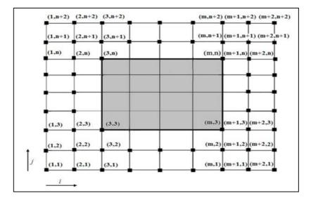
Fig.1. A schematic showing the plate mesh numbering
