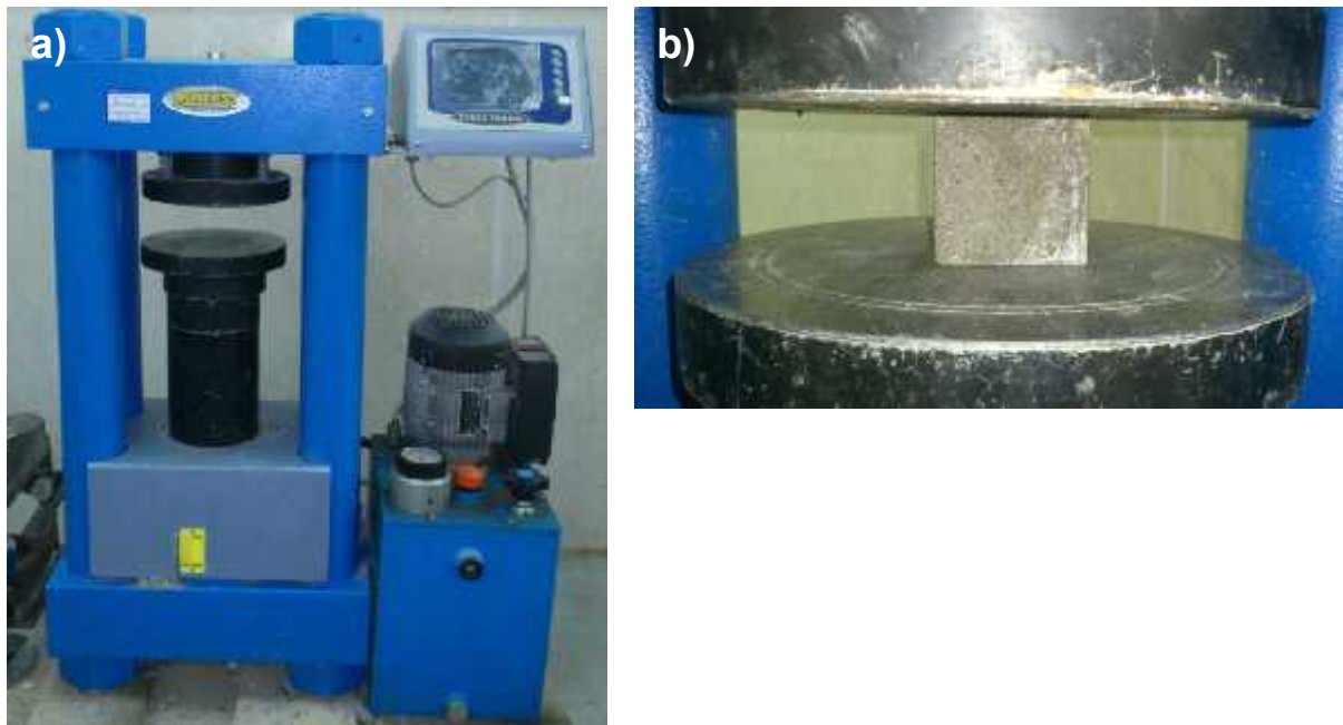
Figure 2: a) Compressive strength test machine. b) Specimen inside the testing machine.
