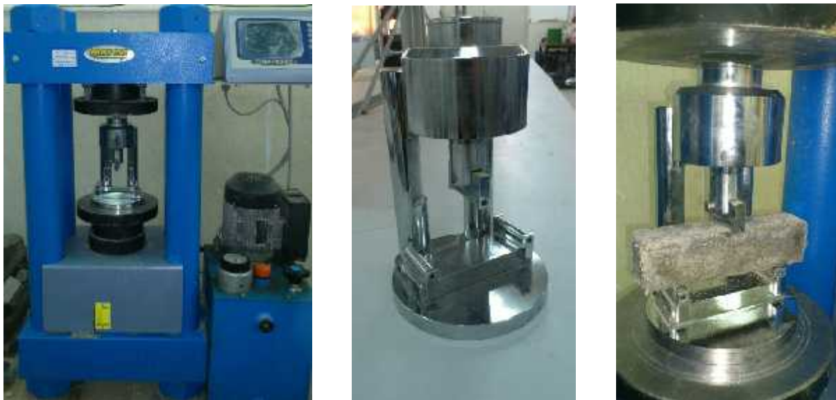
Figure 3: Flexural strength test machine and specimen inside the testing machine.
