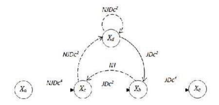
Figure (5) - State Diagrams for convolutional encoder
