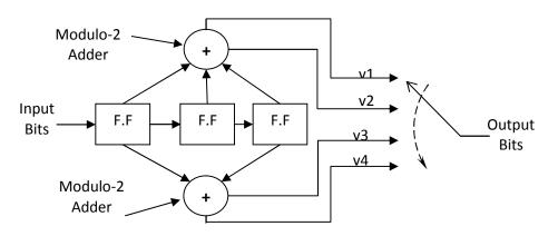
Figure (4) - Block Diagram of Convolutional Encoder with CL= 3 and r = 1/4
