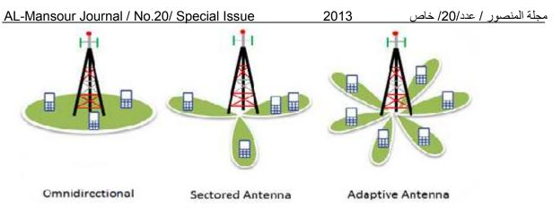
Figure (1) - Base Station Antenna Configuration
