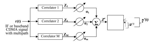
Figure (3) - Block diagram of Rake Receiver.
