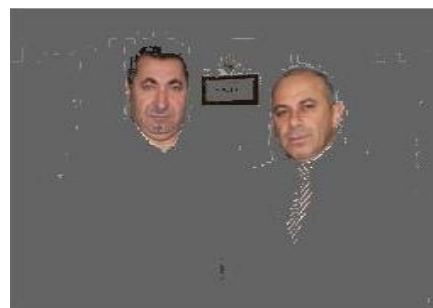
Fig.4 HSI color space skin color condition based segmented image
