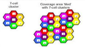
Figure (2): Frequency Re-use use Pattern Repetition
