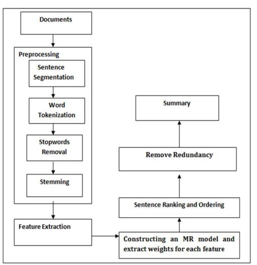
Figure (1) Block Diagram for Proposed MDS
