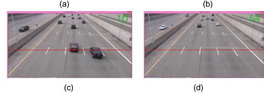
Figure (8) a. The Initial State of the Program Where the Counter is Equal to Zero b. The Counter is Equal to 2 after two cars have passed c. The Counter is Equal to 10 after 10 cars have passed d. The Counter is Equal to 54 after 54 cars have passed
