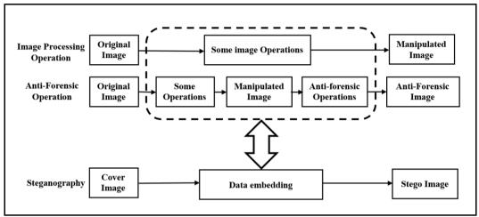
Figure (1): Image processing operations and anti\_forensic operations VS steganography.(some operation in above figure is Contrast enhancement, Sharpening, Spatial Filtering, Lossy compression and Median filtering<sup>[7]</sup>)
