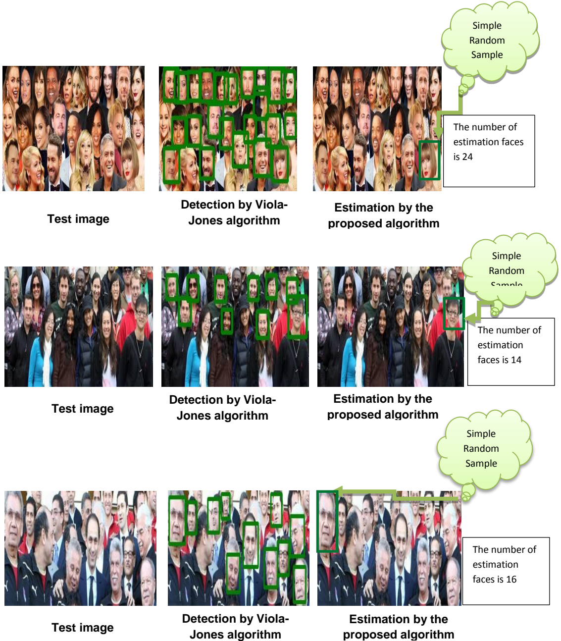
Figure (2): The Detection by Viola-Jones algorithm and estimation by the proposed statistical algorithm of four test Images.
