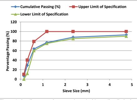
Figure 1. Grading curve for natural sand with grading limits in zone 3.
