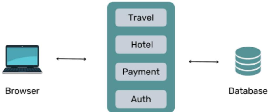
**Figure 1: Monolithic Architecture**
